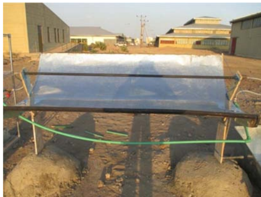
Figure 3. Installed Parabolic Solar Concentrator.
